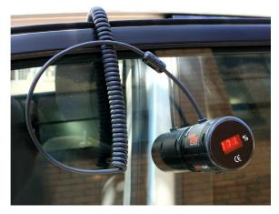
\*For all door windows: The cable MUST be over the door,as pictured, for the magnets to hold. This balances the weight.
