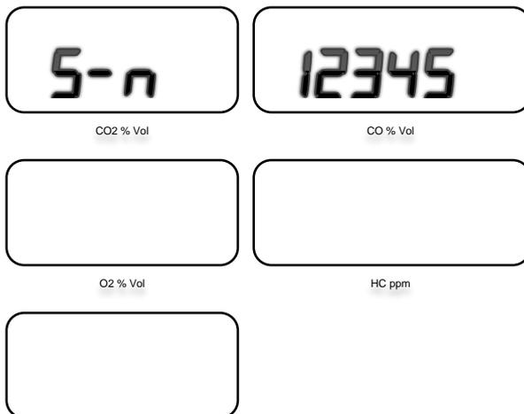
Figure 8 - Device serial no. shown at start-up, reads “S-N 12345”.
