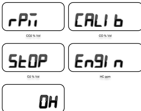
Figure 16 – RPM calibration screen, reads "RPM Calib, Stop Engine".
