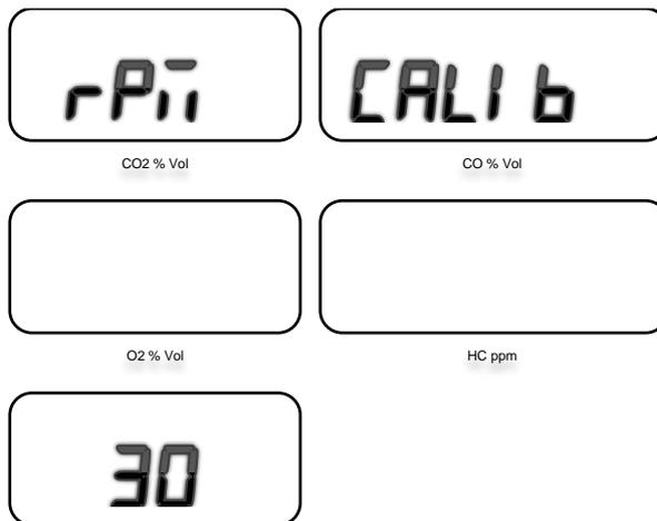
Figure 45 – Screen for rpm calibration
