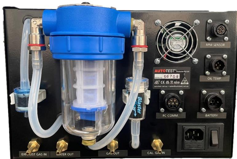
Figure 3. Rear View of AutoGas
