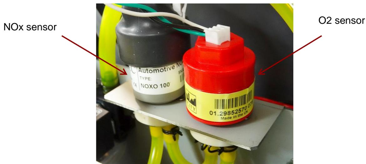
Figure 77 – NOx and O<sub>2</sub> sensors inside the unit
