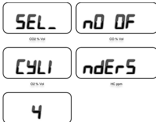
Figure 43 – Screen for entering no. of cylinders
