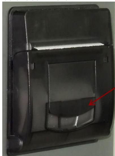
Figure 17 – Built-in Thermal Printer in AutoGas
