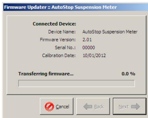
7. The upgrade can take up to 30 minutes to complete. The new firmware will be automatically updated from this point. When the firmware is transferred completely, a message box will appear and the firmware update utility will automatically exit.
