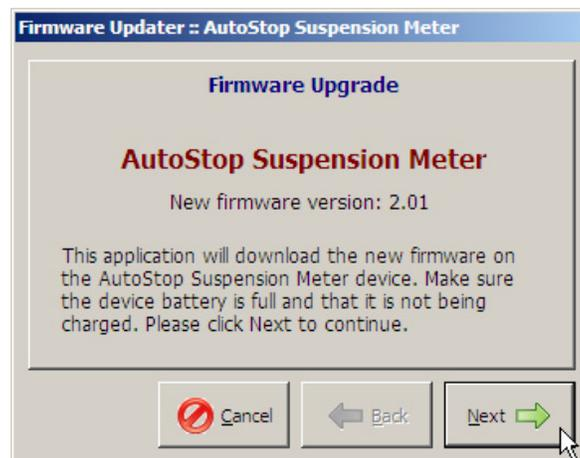
4. After downloading and running the above firmware updater utility, now connect the suspension meter to the PC using the RS232 serial cable or USB-to-Serial cable. Click next when done.
