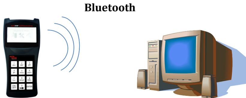
When connecting the Suspension Meter for the first time using the Bluetooth interface, user will need to configure the Bluetooth connection. To configure the Bluetooth connection, open your Bluetooth manager program on your PC and search for Shock##### device, where '#####' is the serial number of the suspension meter.
