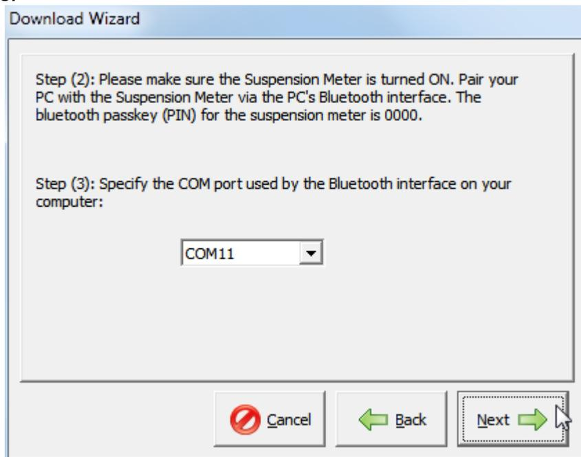
Make sure the suspension meter is ON. Press Next to continue. Once the connection is established, the datalogger software will acquire a list of all tests currently stored on the device.
