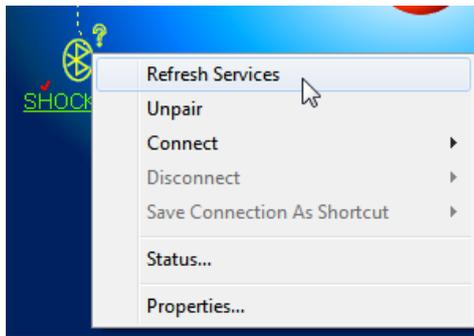
Once the pairing is established, refresh device services and connect using Bluetooth serial port service.
