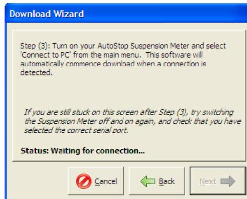
**Step 5:** When you see the above screen on your PC, switch ON the Suspension Meter. When the Main Menu appears, select '**TRANSFER**' by pressing **3** from the keypad on the device. Download will automatically commence once the connection is successfully established.
