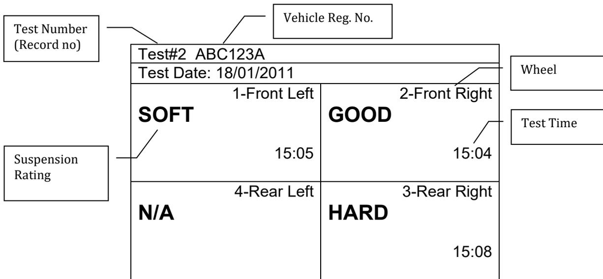
The above screen displays a brief summary of all four wheels of the latest vehicle that is tested. In the above summary screen, the displayed 'N/A' for the 4<sup>th</sup> wheel (Read Left) indicates that 'Not available', or no test was conducted or stored for that wheel.
