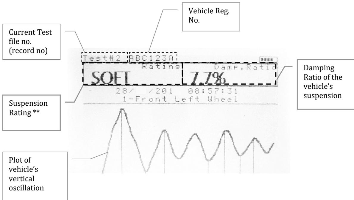
\*\* Suspension rating is evaluated based on Damping ratio., number-of-rebounds, and reference method used (see section 3.6 & 3.7 for more information).
