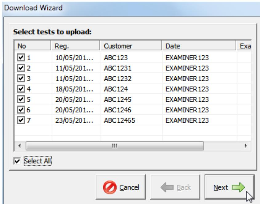
Select the tests that need to be downloaded and press Next. Datalogger software will then download the selected tests.
