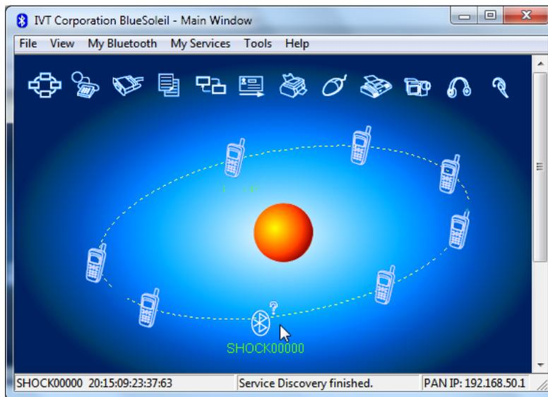
Select the device Shock##### from the list of discovered Bluetooth devices and create pairing.
