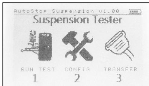
Before starting a test, make sure the device has sufficient (over 30%) battery life. To run a suspension test, select “**RUN TEST**” by pressing ‘1’ from the keypad. The device will show the following list of options on the screen:
