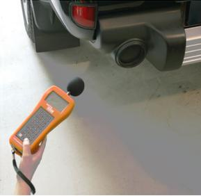
The AutoTest eNoise is a hand-held, stand-alone portable instrument for the measurement and analysis of sound pressure level emitted by stationary vehicles at a nominated engine speed.
