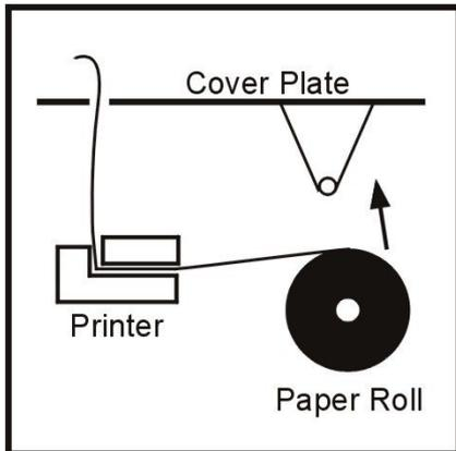
4. Tear off any remaining paper. With the Brake Meter turned on and at the "Ready" mode, press the "P" key on the keyboard to feed any remaining paper through the printer.
