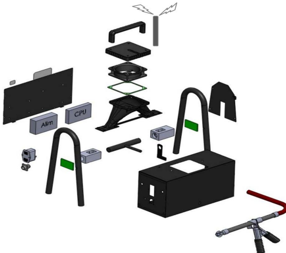
When Auto Smoke is first started, it will go through its initial warmup process. The warmup time should not be longer than 10 minutes over a temperature range of 0-50°C. Once the warmup is complete, Auto Smoke will try to maintain the temperature of the measurement cell at 80°C.
