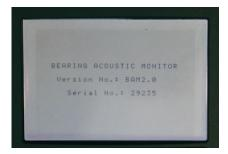
The software version is identified with the "Version No:". The serial no of the unit is also displayed. Wait approximately 5 seconds for all of the software routines to load and to run a self-check.
