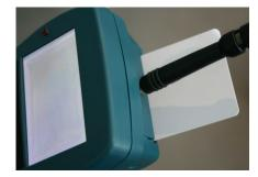
You can save your settings to the smart card by inserting the smartcard as shown above, then selecting *SAVE to SMART CARD* from the menu.
